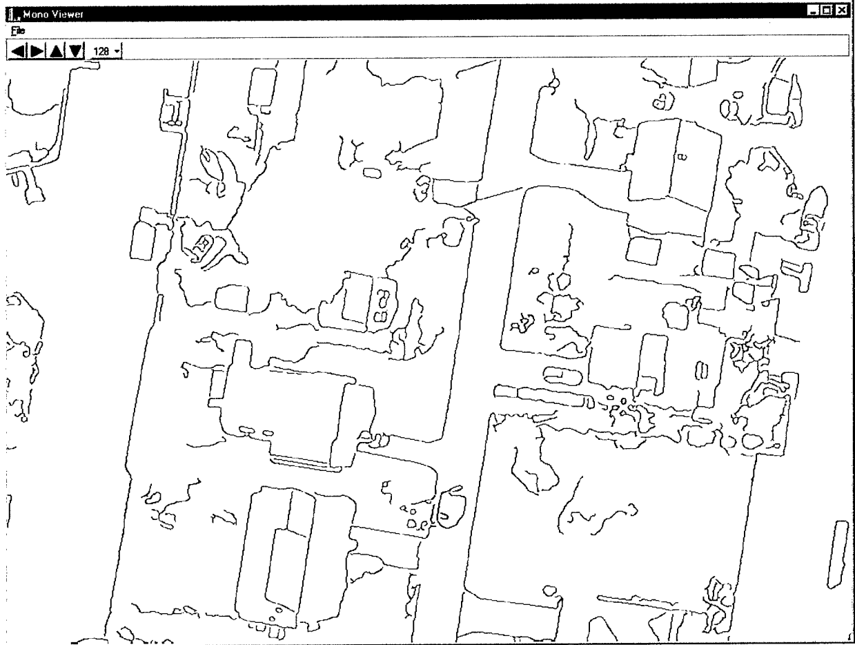
Figure 1: Edge processing result overlaid with the “red” correlation match result
