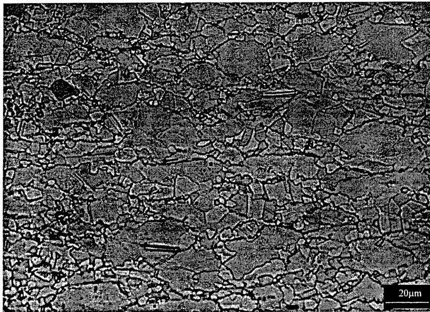
Figure 15: Microstructure of IN-718 after deformation to a strain of 0.69 at 975°C at a strain rate of 10^{-3}\text{s}^{-1} .
