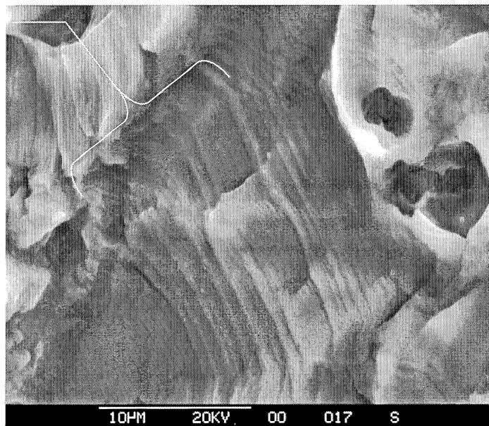
Figure 87 Fatigue Striations from 15E20L, High Magnification
