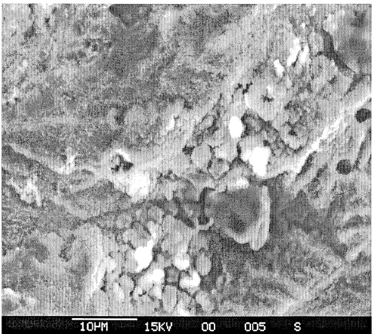
Figure 178 Corrosion on 4C12R
