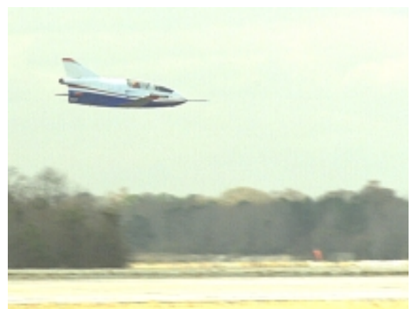
Figure 1-6 JCMD will utilize the BD5-J mini-jet as a cruise missile surrogate
