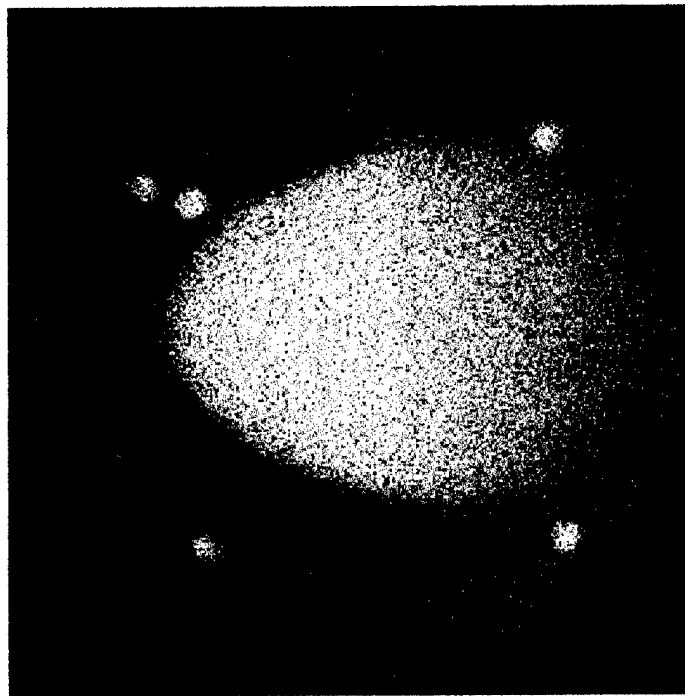
Figure 6. One projection through the phantom. The 5 fiducial markers are clearly visible. The tumor is barely visible.
