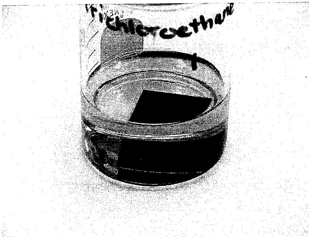
Figure 6. Krylon Interior/Exterior Paint in 1,1,1-trichloroethane (24 h).
