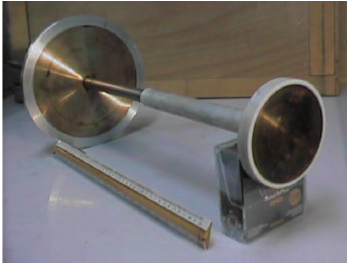
Fig. 2. A general view of the planar cryogenic target, which can be placed at a chosen distance from the PF electrode outlet. When liquid nitrogen is pumped through the inner tubes, and a small amount of heavy water ( D_2O ) is injected into the experimental chamber with an auxiliary valve, the target plate can be covered with a heavy-ice layer. To reduce the consumption of D_2O there is installed an external thermal shield.
