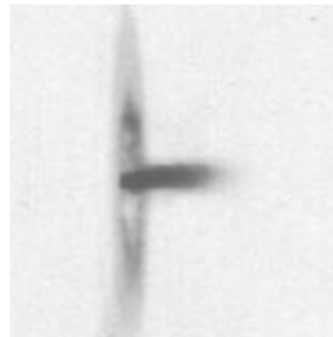
Fig. 7. Soft X-ray pinhole pictures, which were taken with a pinhole camera, for several discharges performed in the PF-360 machine equipped with the planar cryogenic target. It can easily be seen that the placement of the planar cryogenic target did not influence the X-ray emitting plasma region noticeably.
