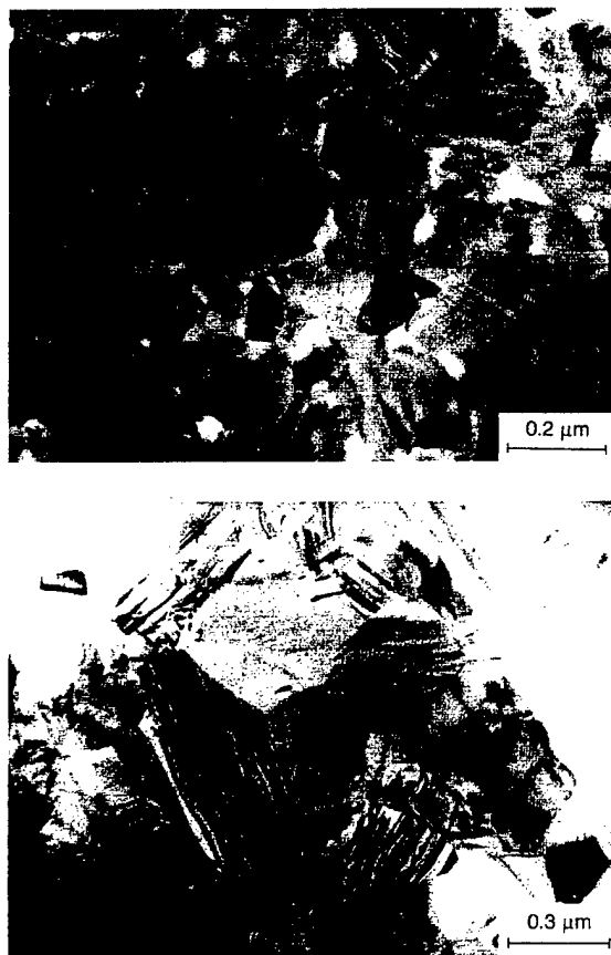
Fig. 4. TEM micrographs showing the grains in a near-stoichiometric UF-HM fiber.
