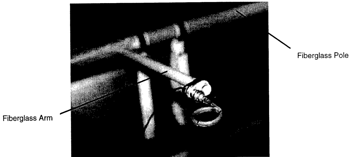
Figure 5. Magnetic Field Loop Sensor
