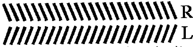
Figure 4: Two states (R, L) of louver filter. Looking up from this caption toward the filter, in the R state the bias favors the right eye, in the L state it favors the left eye.
