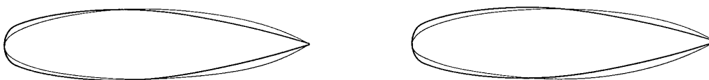
Fig. 17 - Shape of the modified airfoils for the untwisted (left) and twisted (right) wings
