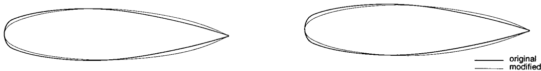
Fig. 22 - Shape of the modified airfoils for the untwisted (left) and twisted (right) wing, with l.e. radius constraint
