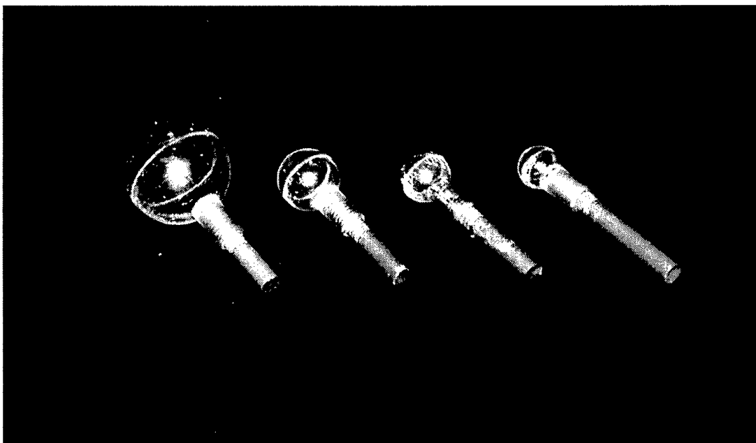
Fig. B Some of hollow plastic spheres used to simulate lesions. Several hollow plastic spheres, with diameters ranging from 4 to 28 mm, were procured to simulate lesions. Each sphere can be mounted to the base of the breast phantom with a thin plastic rod. A wide variety of single/multiple-lesion scenarios can be modeled.
