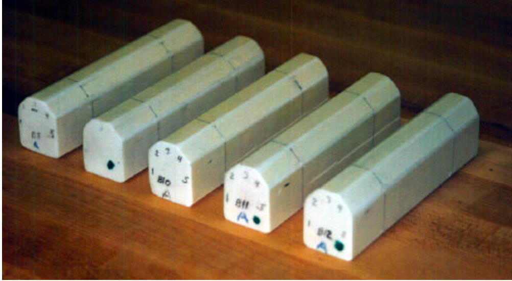
Figure 24 - Five wire-artifact, five-sided, RFC-style, MACOR® substrate calibrations blocks are shown.
