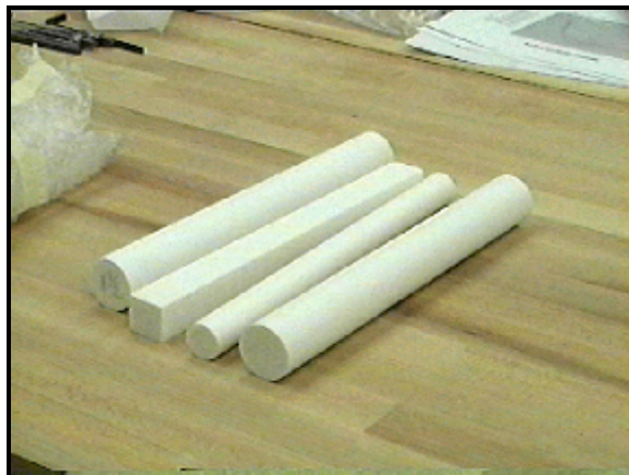
Figure 3 - MACOR ® stock used for substrate material for surface calibration blocks and RECHII inserts.
