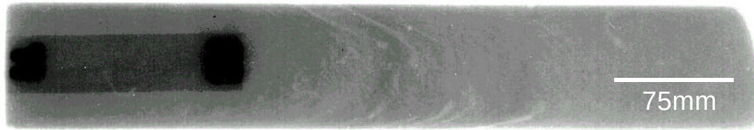
Figure 1- X-ray radiograph of a cross-section of forged 3-95 showing macrosegregation-related banding (dark rectangular area is used to characterize X-ray sensitivity).
