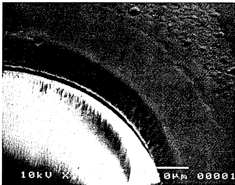
Figure 3: Smoothing of the cathode edge in the conformal mask technique. The illuminated region extends 10 \mu\text{m} past the edge of the well.
