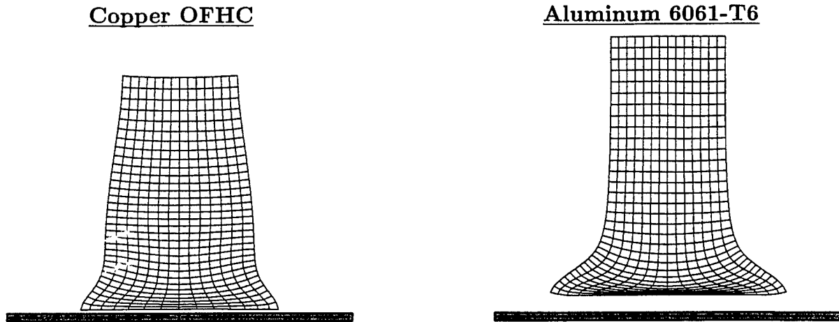
FIGURE V.6.2 Impact of a circular bar. Lagrangian solutions for the Copper OFHC and Aluminum 6061-T6 bars.
