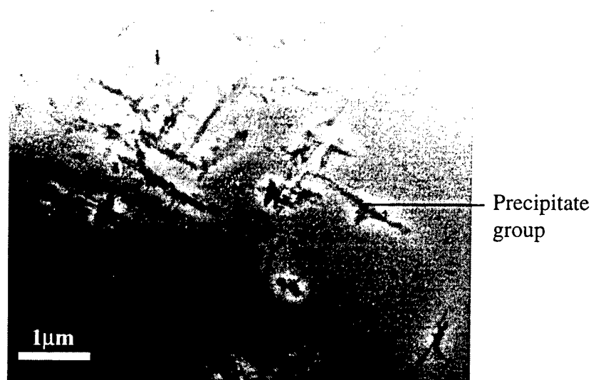
Figure 2 Many-beam bright-field transmission electron micrograph showing the typical distribution of precipitate groups within a (Nb) dendrite. Each group consists of many precipitates. Beam direction \mathbf{B} is close to \langle 001 \rangle_{(\text{Nb})} .
