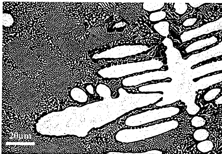
Figure 1 Backscattered Electron (BSE) scanning electron micrograph showing a transverse section through the as-DS binary composite. The (Nb) dendrite is surrounded by a eutectic mixture of \text{Nb}_3\text{Si} and (Nb). (Nb) is the lighter phase.
