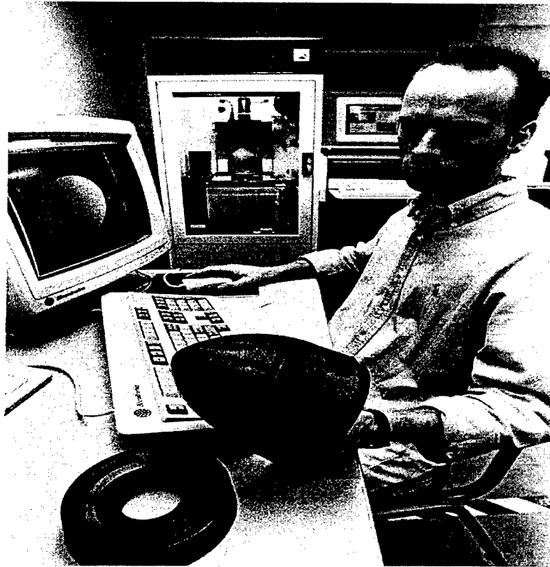
Figure 12: Rapid prototyping of the SRAW warhead in the Rapid prototyping facility; SLA-250 in the background
