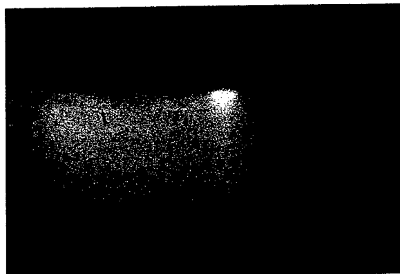
Fig. 7. Picture of the fluorescence emission at the output facet of the single mode waveguide
