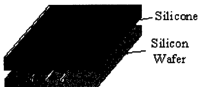
Step 3: Pour GE RTV 31 silicone compound onto silicon mold. Allow to cure, then remove.
