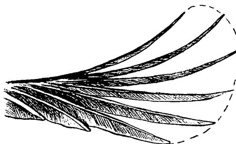
Fig. 26. Theoretically, the induced drag can be minimized by an infinite number of winglets. In this case, the tip vortices would form a continuous vortex sheet along the outline of this configuration. Certainly, such a configuration can not be built in practice. But a similar wake configuration may be achieved by a lifting line shaped like the enveloping curve and by an appropriate arrangement of the circulation distribution along that line
