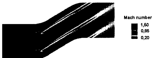
Figure 8: 2D Navier-Stokes – k-\epsilon turbulence model – Mach number contours
