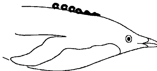
Fig. 11. Schematic graph of a rare high-speed video picture showing the development of ring structures in the boundary layer of an Adelie penguin
