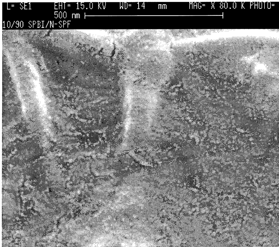
Figure 43. SEM micrograph of the NPSF/SPBI (90/10 w/w) molecular composite.
