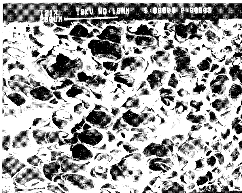
Figure 27. SEM photo of microcellular P2VP foam with low density.
