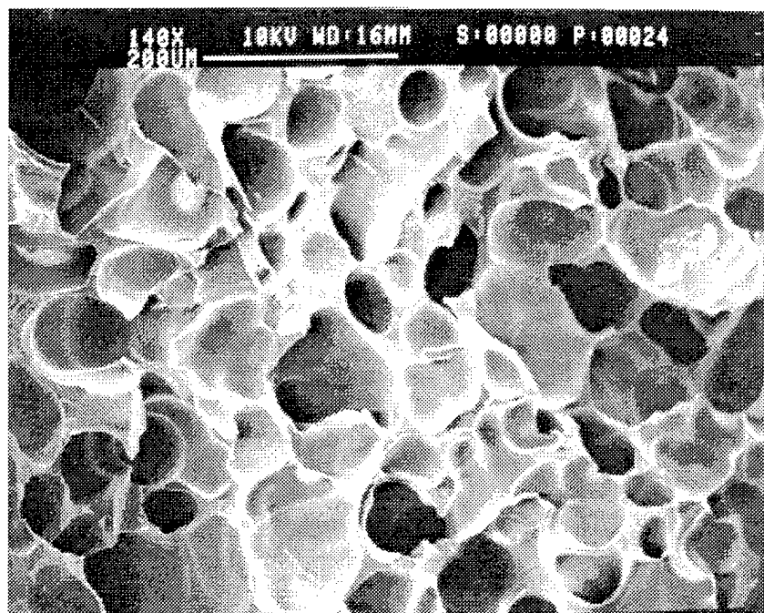
Figure 26. SEM photo of microcellular P2VP foam with intermediate density.
