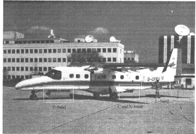
Figure 1. The E-SAR system mounted on a Do-228 aircraft. The antennas of the multi frequency SAR system are depicted in the yellow
