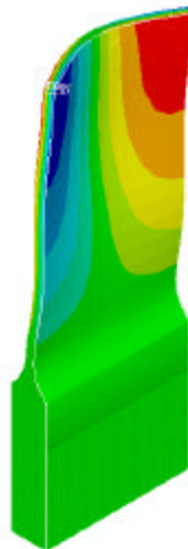
FIGURE 102. The 5 KHz 1-2s Mode of a Simple Cantilevered Plate
