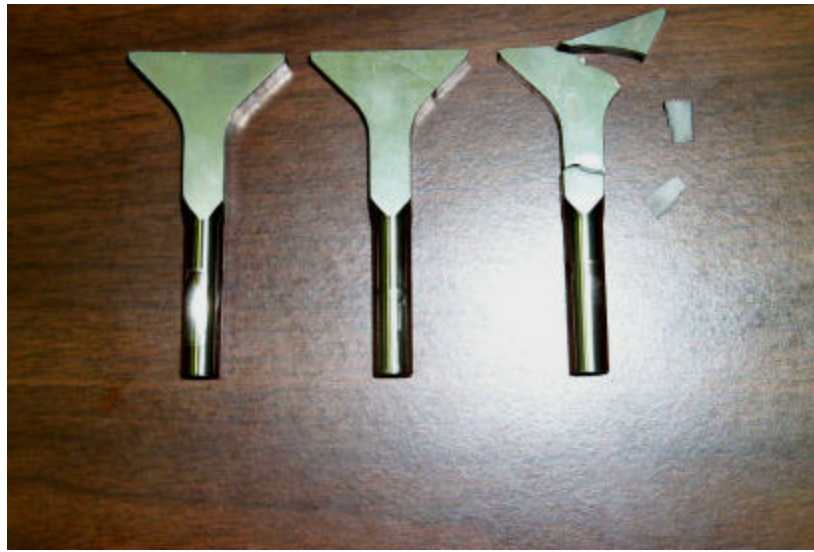
FIGURE 22. Different Levels of Damage In Dovetail Fatigue Specimens
