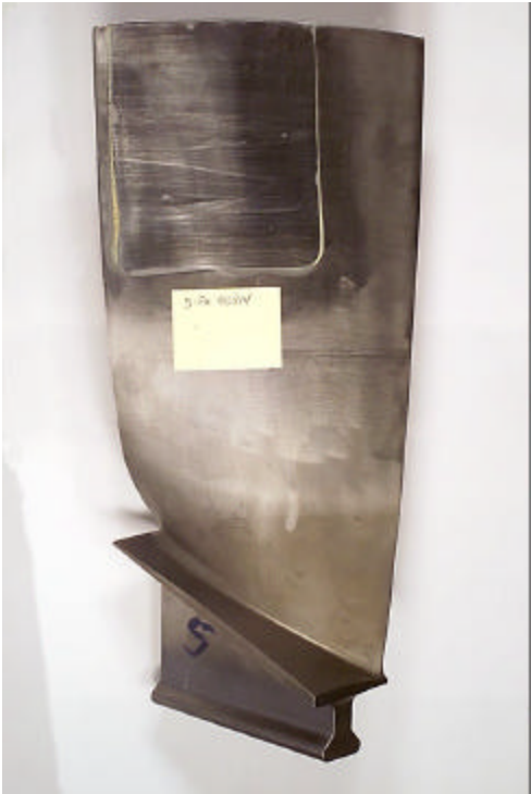
FIGURE 99. Blade 5 with Damping System Installed
