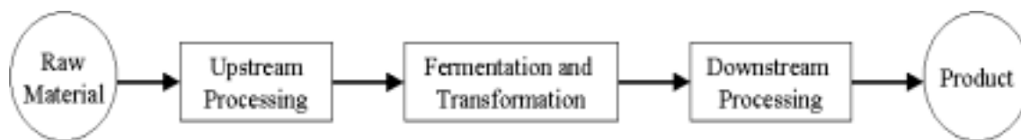
Figure 4. Notional Industrial Microbiological Process
