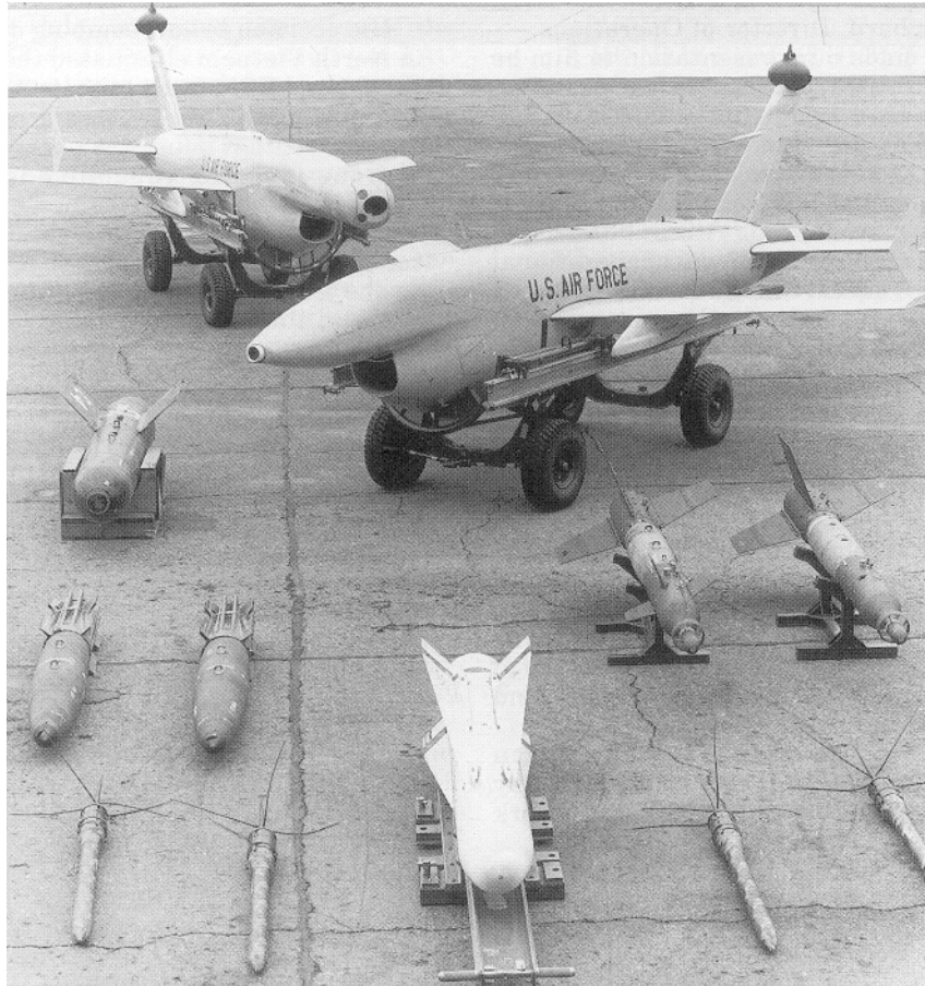
Figure 7. A Ryan BGM-34A pictured with some of the weapons it carried, which included Maverick and Stubby Hobo missiles, and Mark 81 and 82 iron bombs. A BGM-34B is pictured in the background. (Courtesy of Barnes and Noble Publishing)
