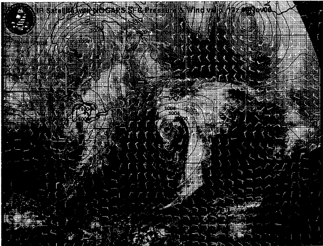
Figure 1. Fused GOES satellite and NOGAPS product for the North Atlantic Ocean, 1900 UT, 09 November 2000, produced by NLMOC-Norfolk using WSI software.
