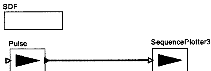
FIGURE 16.6. A model that plots the values of a signal. 256 iterations must be executed to plot the entire signal.
