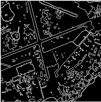
Figure 13: Edge images obtained from application of Canny edge detector to segmented images.
