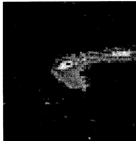
Figure 5: Thermal image of a shear band ahead of a crack tip loaded under Mode II conditions. The image is 1.92 mm x 1.92 mm. The maximum temperature rise associated with the shear band formed at K_{II} = 77.3 \text{ MPa}\sqrt{\text{m}} was \sim 0.5 K [9].
