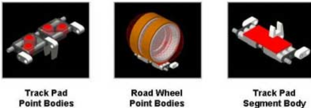
Figure 4. DADS Point-Segment contact force element "Point" and "Segment" bodies.
