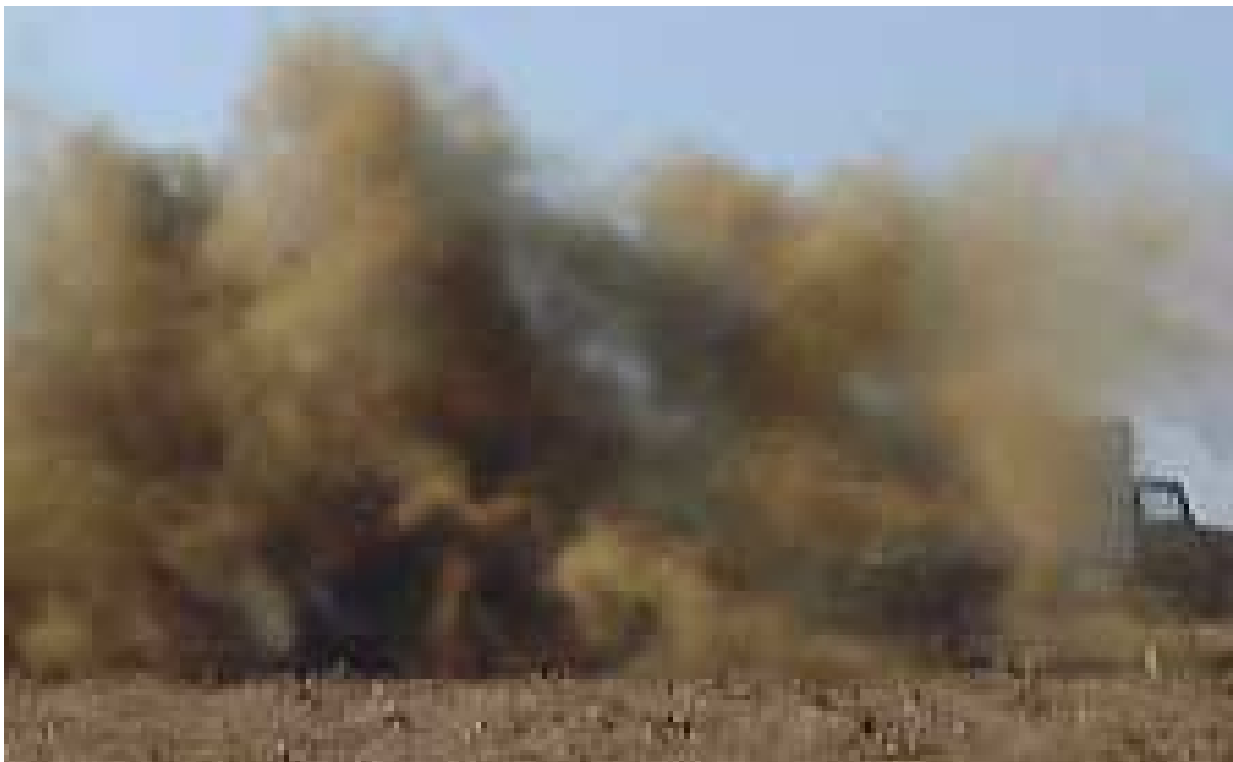
Figure 10. Continuous curtain produced from a 3.3-second firing interval.
