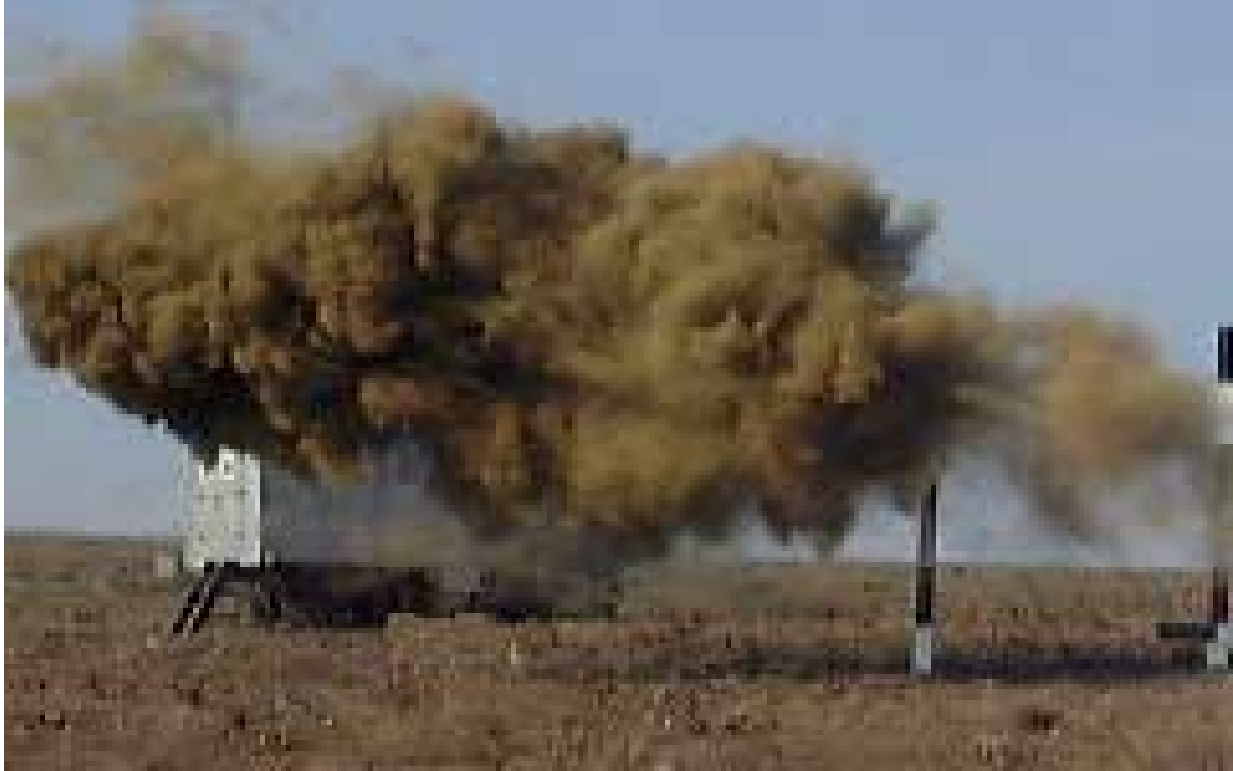
Figure 9. Composite puff produced from a single salvo, 6-chamber quick burst.
