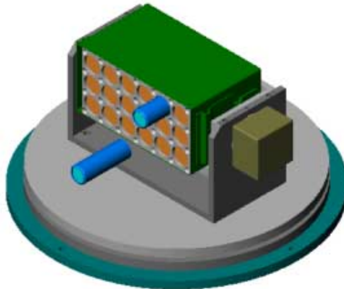
Figure 12. Adaptation of smoke pot as a launcher for projected screening cartridges.
