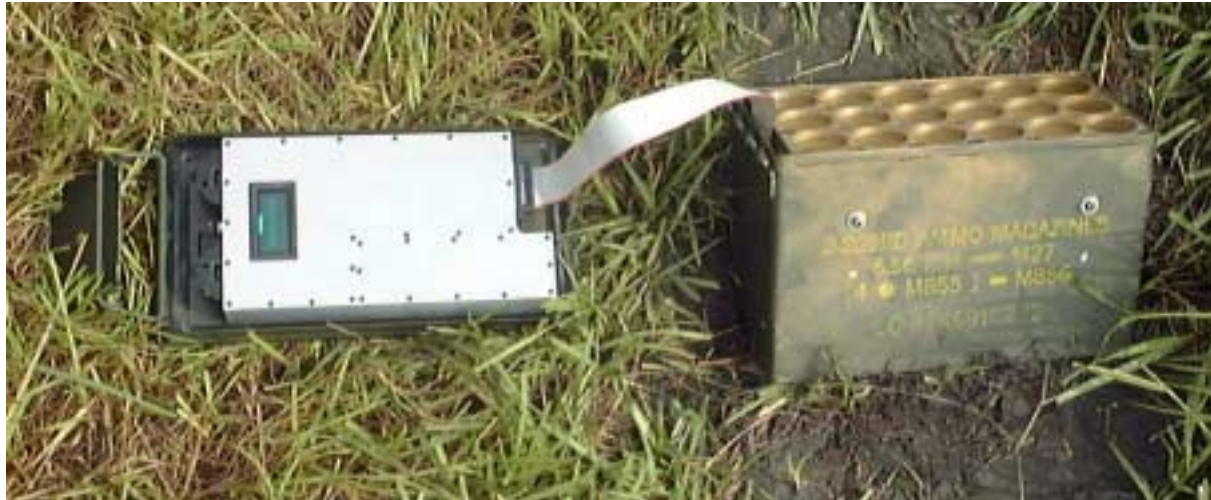
Figure 5. Smoke pot unit emplaced and ready for function.
