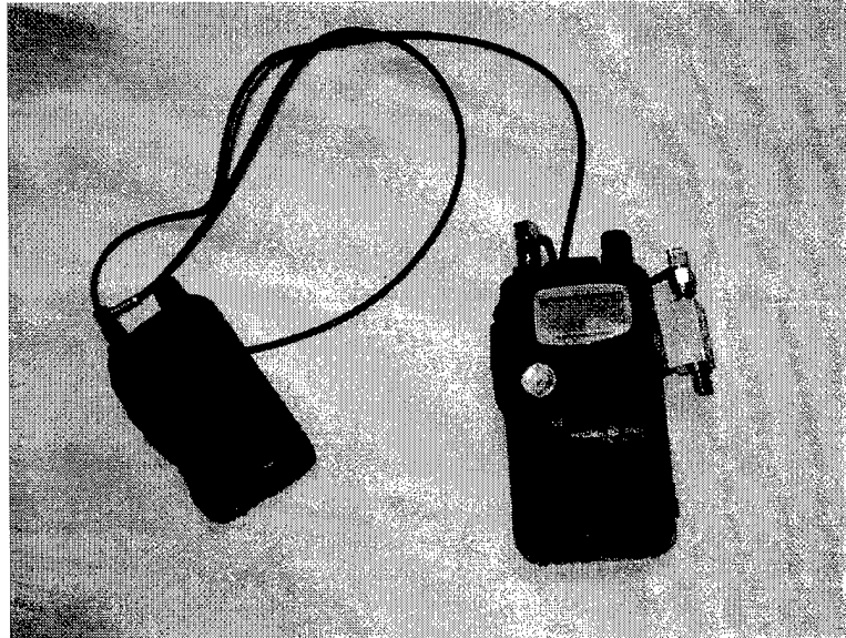
Figure 4.3-2 Major components of brassboard soldier radio
