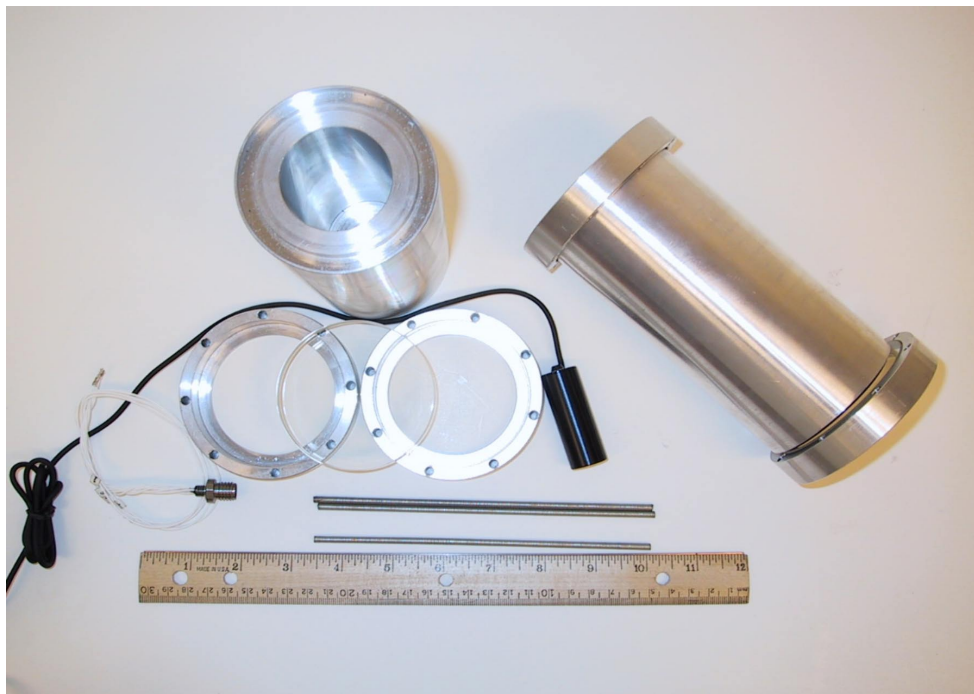
Photograph MED-23: Camera Housings, with Contents, Glass Front, and Connector Hardware.
