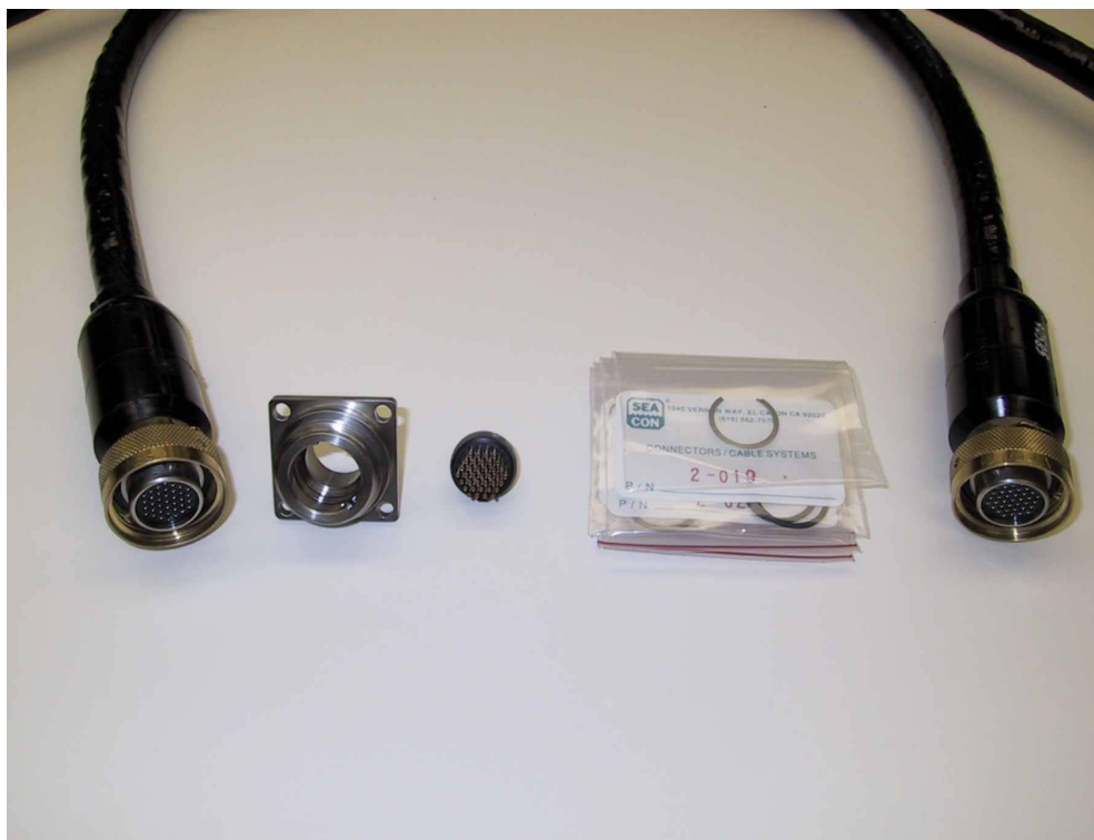
Photograph MED-30: High-Density Deep-Ocean Underwater Cabling and Pressure Vessel Fitting.
