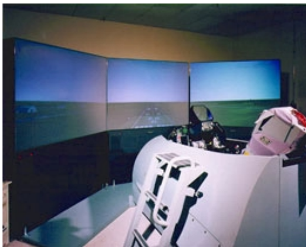
Fig 5.10 Providing an immersive experience through the use of peripheral visions. (a) An artist's impression of the Infinity Wall. (Image by Jason Leigh, Electronic Visualisation Laboratory, University of Illinois and Chicago). (b) Multiple Screens configured as a flight simulator, showing a landing on an aircraft carrier. (Danish Air Force)
