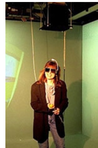
Fig 5.20 (a, above) Projectors present stereographic imagery on the walls of the CAVE. (b, below). A user in the CAVE
