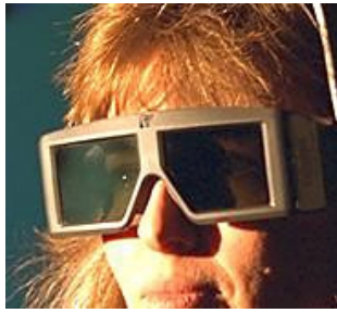
Fig 5.9 (Electronic Visualization Laboratory, University of Illinois at Chicago) Shutter glasses for stereo viewing. Each eye is allowed to see the display on alternate frames. Shutter glasses are available from StereoGraphics
