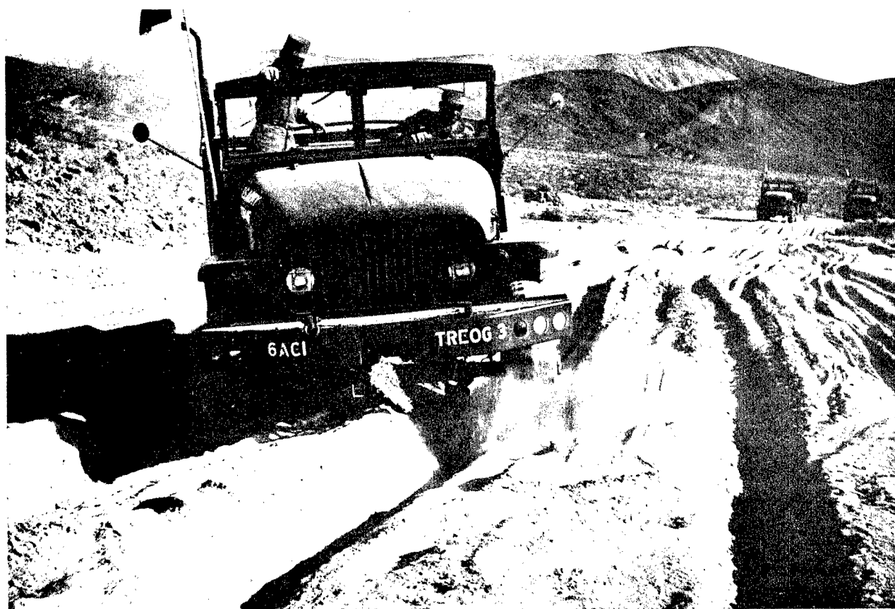
FIGURE 9. TRUCK CONVOY ON SOFT SAND. AS A PART OF THE USA TREOG OPERATION DESERT TRAINING II THE TREOG TASK ELEMENT CONDUCTED TRAINING IN DESERT DRIVING. THE TREOG CONVOY SHOWN ABOVE IS TRAVELING THROUGH A SOFT SAND AREA IN THE MOJAVE DESERT AT CAMP IRWIN, CALIFORNIA. THE LEAD TRUCK COMPACTS THE SURFACE WITH ITS TIRES AND THE REMAINING TRUCKS FOLLOW IN ITS TRACKS.
