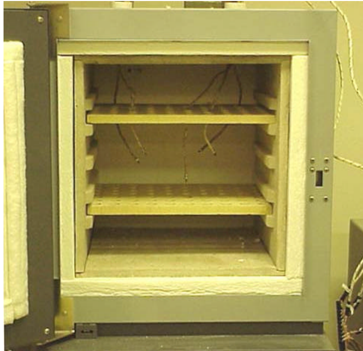
Figure 14. Muffle furnace with five high-temperature J-type thermocouples.
