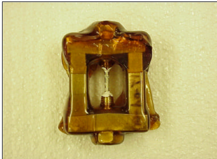
Figure 27. Failure of an alternate immersion specimen due to stress corrosion cracking (SCC).
