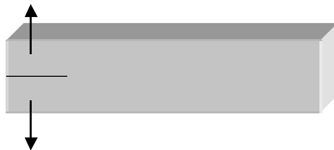
Figure 5. Schematic of double-cantilever beam specimen indicating the direction of loading and crack propagation.
