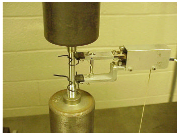
Figure 19. One-inch extensometer mounted on a tensile specimen.
