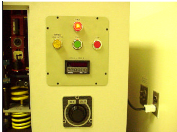
Figure 23. Cycle counter on fatigue apparatus.
