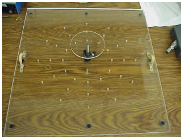
Figure 14. Lucite base with holes drilled for positioning.
