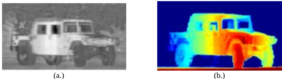
Figure 9. (a.) Intensity image of a HMMWV at 60 m range reconstructed from MFOV ( 12.6^\circ ) MSTIL data. (b.) Range image of a HMMWV at 60 m range from MFOV MSTIL data (original in pseudo-color).
