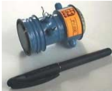
Figure 19. Commercially available Compact Streak Tube. Streak Tube Dimensions: 8.0 cm (3.15 inches) long by 6.5 cm (2.56 inches) in diameter.
