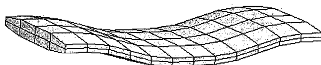
FIGURE 61. FINITE ELEMENT MESH FOR A SECTION OF CRIMPED YARN
