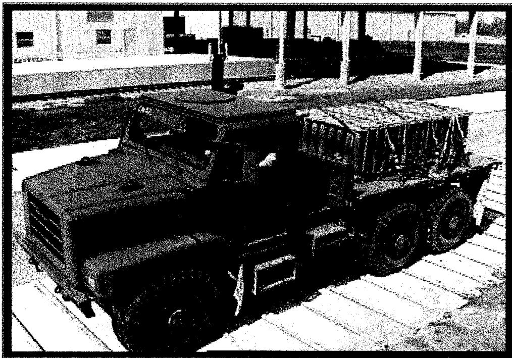
Washboard test of MK-25 with 155MM Separate Loading Projectiles
