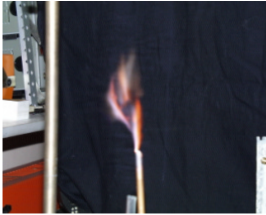
Fig.4b. HF streamer discharge in airflow ( M \sim 0,4 , P_{st} \sim 1 Bar) without propane injection (a), with it (b). Airflow and propane injection directions are from down side up of the photo to its topside.
