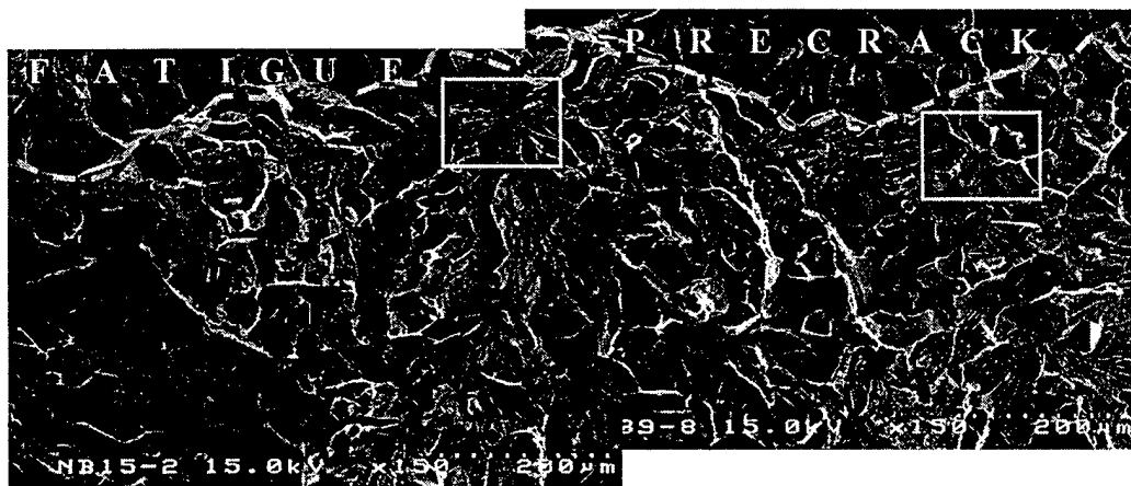
Figure 2. Fracture Surface Montage of an \text{Nb}_{\text{CP}} 40\ \mu\text{m} Fatigue-Precracked Charpy Specimen Tested at -196^{\circ}\text{C} . Apparent Cleavage Fracture Nucleation Sites are Shown Inside the Boxes
