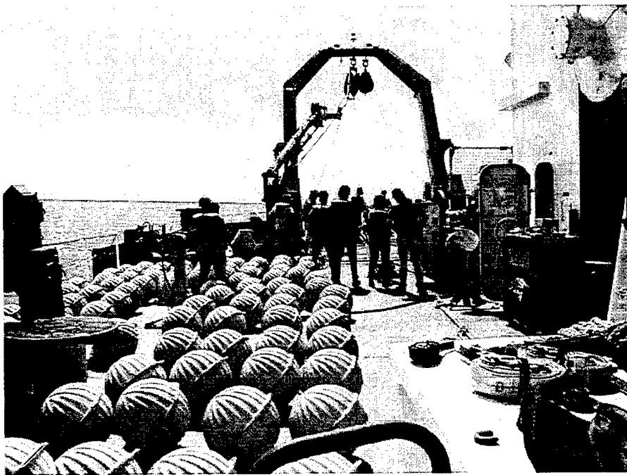
Figure 42: Eighty-one glass balls in hard hats stowed on deck for deployment.
