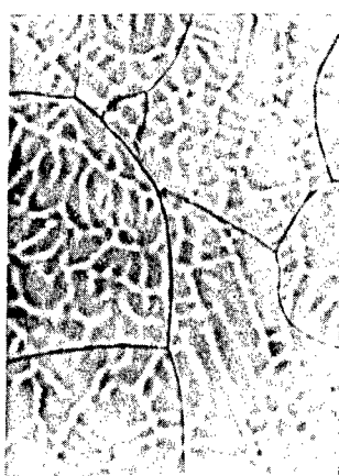
(e) As-welded and then aged 10 hours at 2000° F and 10 hours at 2200° F.
