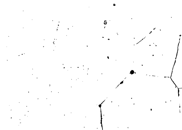
(a) Solution-treated 1 hour at 3000° F.
