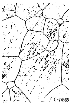
(f) Solution-treated, heat-treated, and then aged 10 hours at 2000° F.
