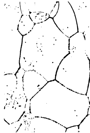
(a) Solution-treated 1 hour at 3000° F.
