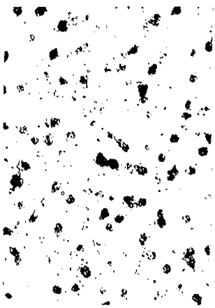
(d) As-welded and then aged 10 hours at 1800° F and 10 hours at 2200° F.
