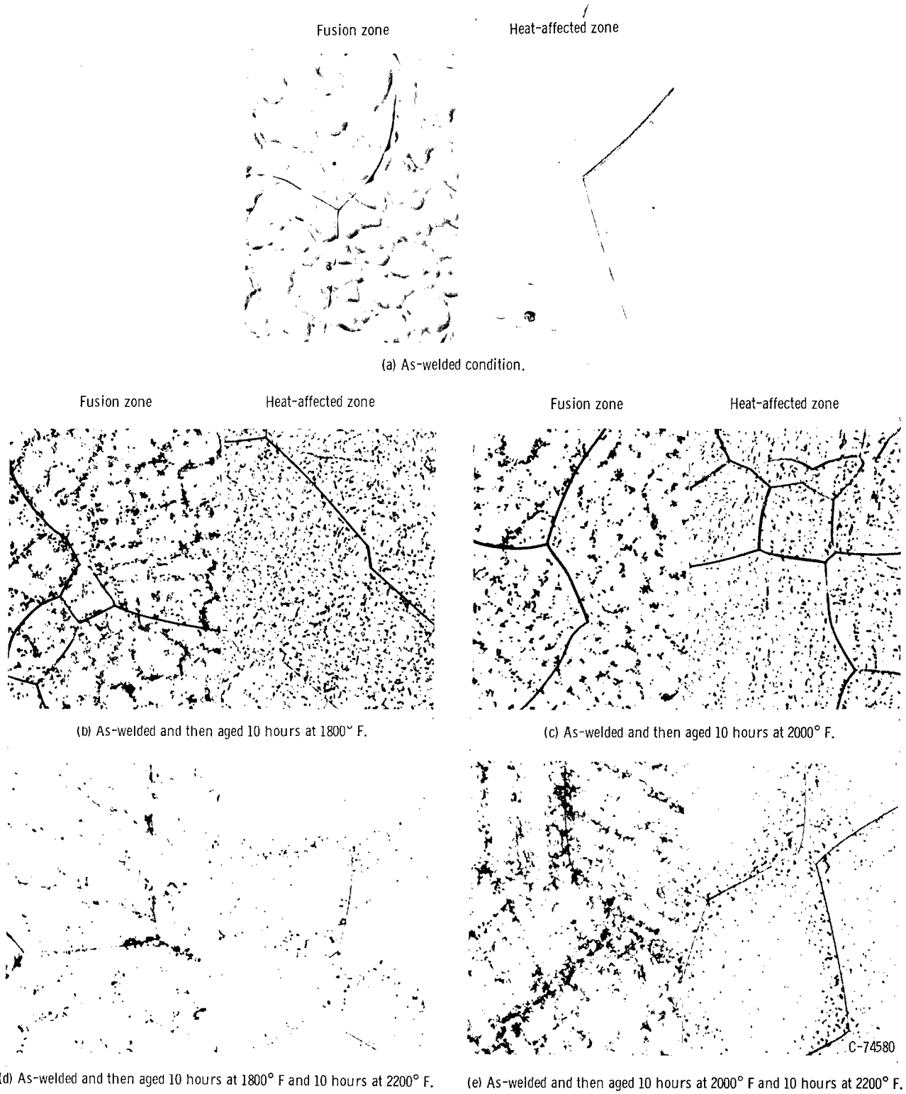
Figure 15. - Microstructures of gas tungsten-arc welded T-222 sheet in as-welded condition and after 10-hour aging at various temperatures. Etchant, nitric acid and hydrofluoric acid. X1000. Reduced 50 percent in printing.
