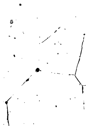
(b) Solution-treated 1 hour at 3000° F and then heat-treated 1 hour at 2500° F.
