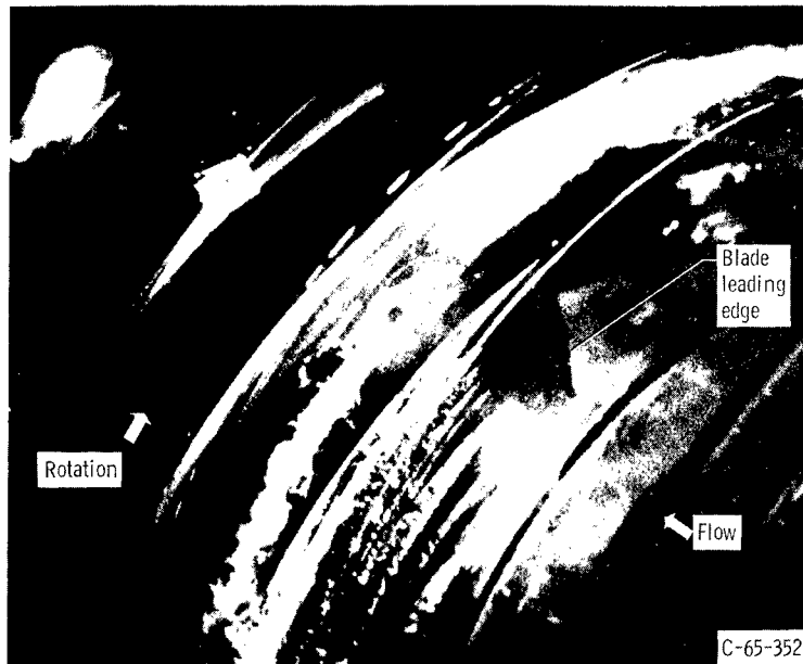
Figure 10. - Blade surface cavitation appearing in streamer form.
