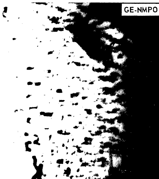
B. UOX + MgO-grade BeO irradiated at 900°C to 1.1 \times 10^{21} nvt (Neg. J-274)
