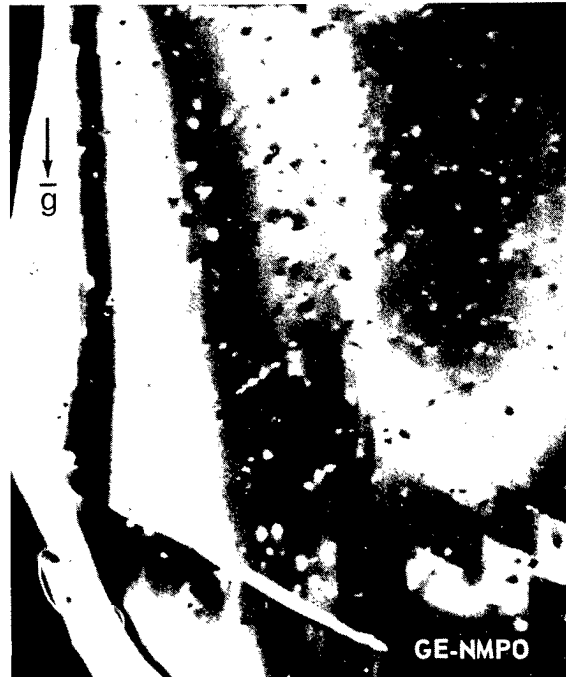
d. Dark field micrograph, \bar{g} \parallel [00.2\bar{1}] . (Neg. J485)
