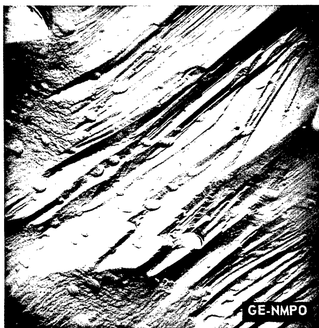
Fig. 3.10 – Intragranular gas bubbles on cleavage surface (Neg. 784C, 7500X)
