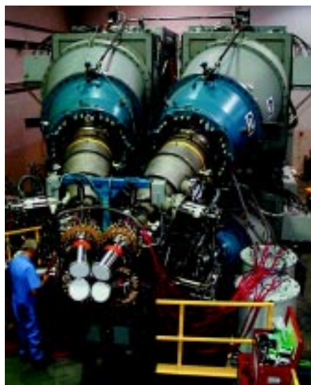
The Decade Radiation Test Facility (above) and X-ray quad (left) simulate radiation effects of a nuclear explosion.
