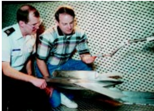
Unmanned combat air vehicle weapon separation test in 4-foot transonic wind tunnel
