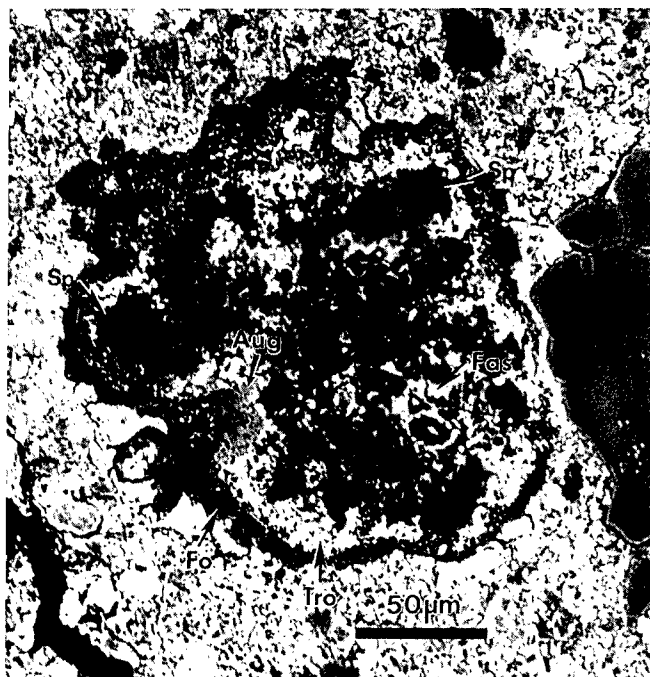
Figure 8. Back-scattered electron microscope image of a CAI from the Bells CM carbonaceous chondrite. It is a nodular spinel-pyroxene CAI that consists of an irregular core of spinel (SP) intergrown with the pyroxene minerals, fassaite (Fas) and augite (Aug), and the sulfide mineral, troilite (FeS). A narrow mantle of forsterite (Fo) rims the inclusion. By courtesy of Adrian Brearley (University of New Mexico). Reprinted from Geochimica et Cosmochimica Acta , 59, A.J. Brearley, Aqueous alteration and brecciation in Bells, an unusual, saponite-bearing, CM chondrite, 2291–2317, copyright 1995, with permission from Elsevier Science.
