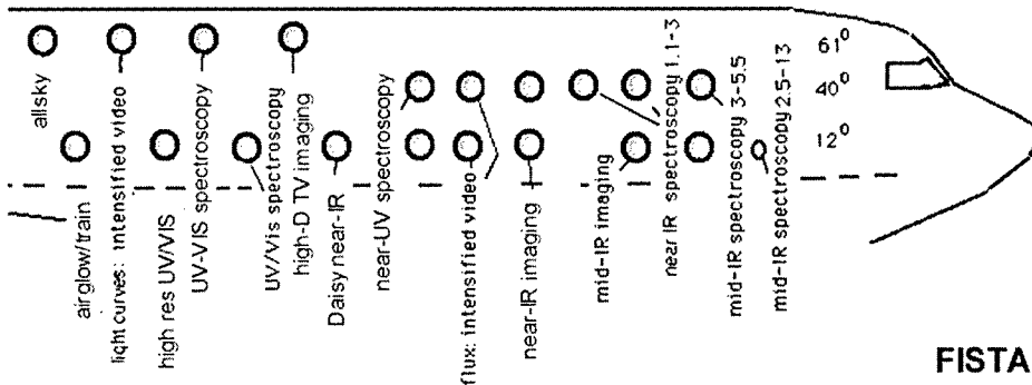
Figure 3. Relative position of instruments on-board FISTA.
