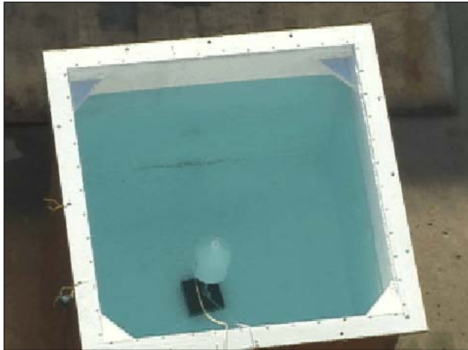
General Dynamics – Ordnance and Tactical Systems (GD-OTS) Fragment Recovery Water Tank
